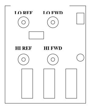
Figure 2: PCB Layout and Trim Pot Location
